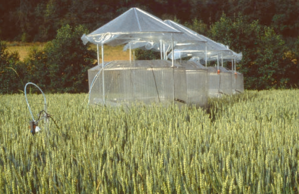
Figure 2. An open-top chamber is a transparent plastic cylinder, which is provided with air through a fan that either filters off or adds pollution. Here, spring wheat is exposed to ozone at the experimental station at Östads säteri, 40 km northwest of Gothenburg. Photographer: Håkan Pleijel
